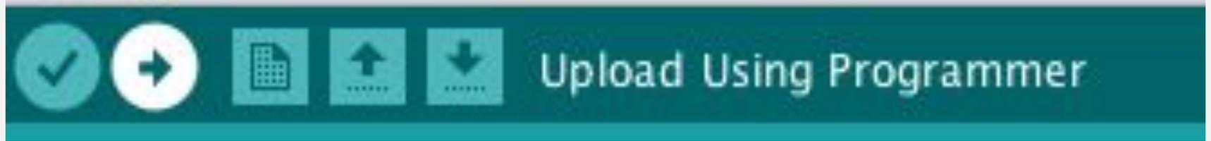
This will automatically check and verify the code and upload the code to Otto.
